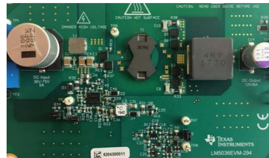
LM5036 EVM fsw = 400kHz 36V-75V / 12V 100W design
