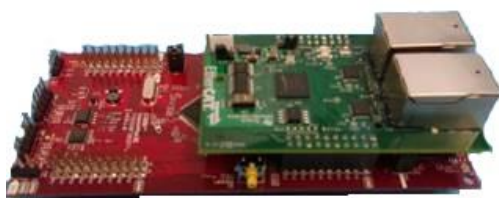
Figure 10. Stacked F2837x LaunchPad and EtherCAT BoosterPack
