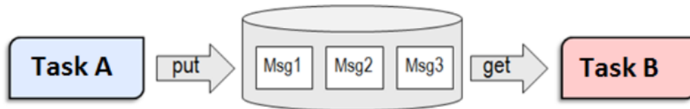
Figure 3-4. Queue Messaging Process
