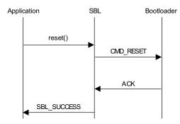
Figure 12. Sequence Chart for SBL Function Reset
