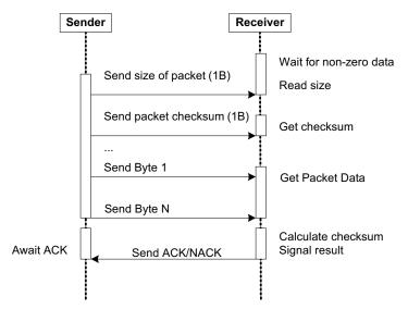
Figure 2. Sequence Chart for Send and Receive Protocol
