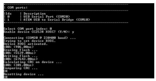
Figure 5. Successful Execution of the CC2538 Example Application
