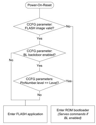
Figure 1. Simplified Flowchart for Entering Bootloader (CC26xx)
