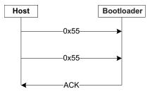
Figure 3. Sequence Chart for Connection Initialization
