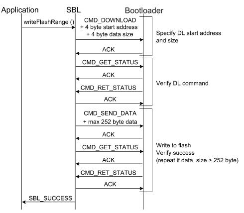
Figure 10. Sequence Chart for Flash Write
