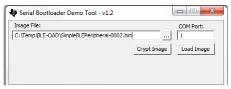
Load and run the OAD Manager application into a separate CC254xEM on a SmartRF05 board which is connected via a serial cable to the PC running the SBL Demo tool. The OAD Manager application can be found here:
