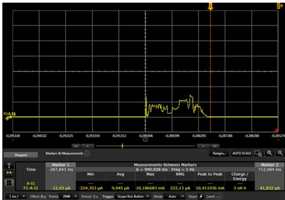
Figure 31. Connection Event, Marker #1 Placement
