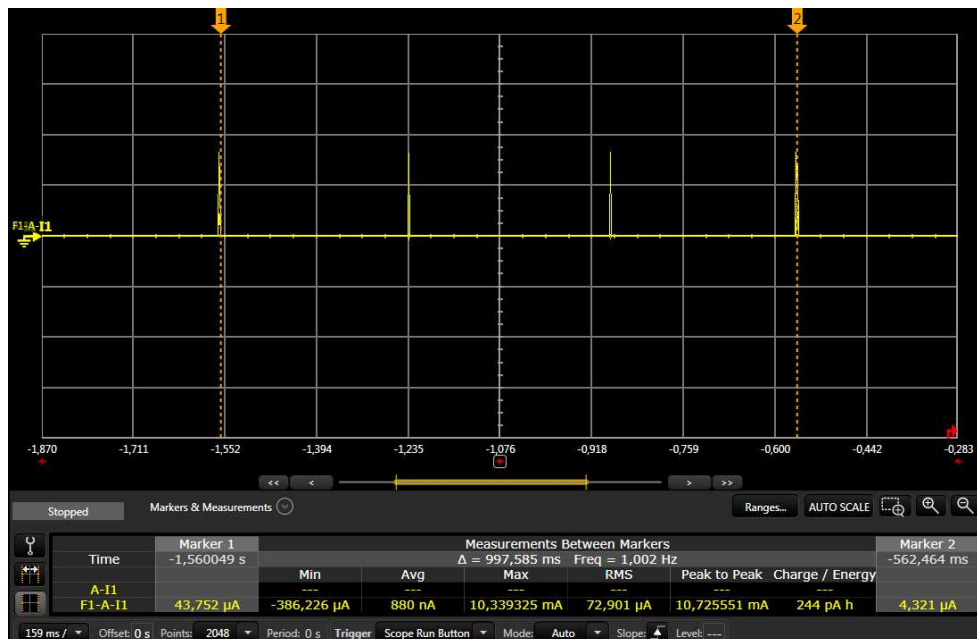
Figure 30. Measuring Standby Current During Connection
