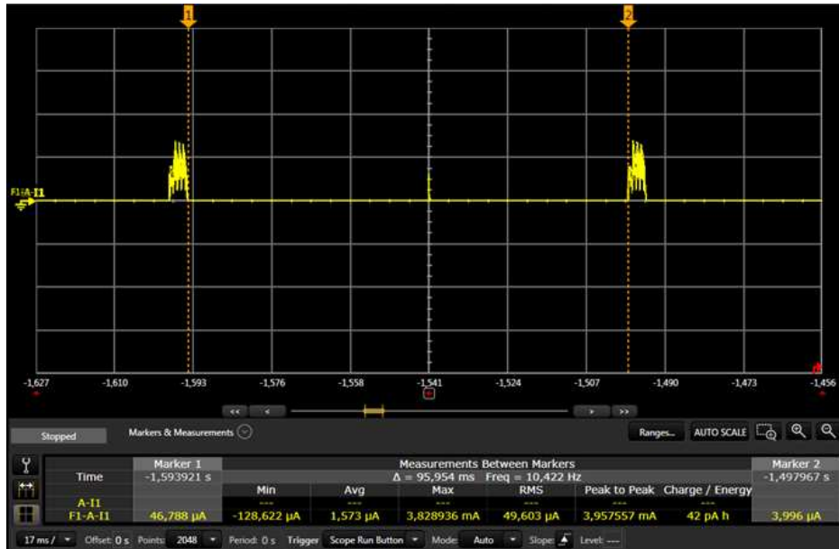
Figure 29. Measuring Standby Current During Advertisement
