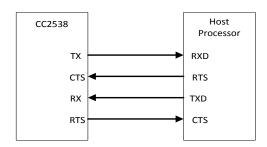
Figure 11 RTS/CTS Flow Control Connections
