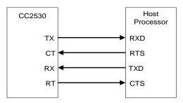
Figure 16 RTS/CTS Flow Control Connections
