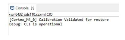
• From this point you can send the configuration file (.cfg) over UART (using the GUI, terminal emulator, etc...) and the device will begin chirping
