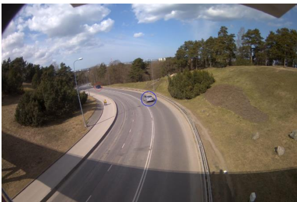
Figure 27. A situation where a track belongs to vehicle A does not exit the defined range on time, and causes mix-up with the track belongs to vehicle B
