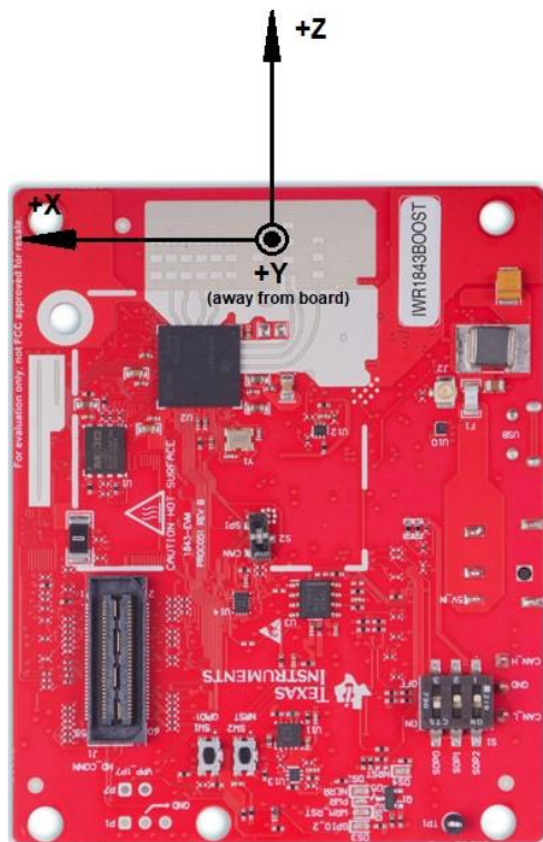
Figure 25. EVM sensor position with respect to X, Y, Z orientation axes
