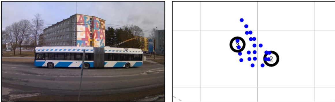
Figure 28. Two tracks for a single object, caused by too small dimension limits
