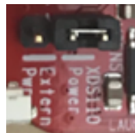
Figure 22. Default XDS110 Power Jumper Setting
