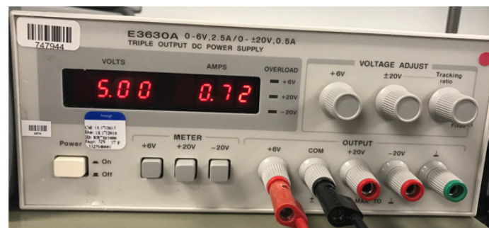
Figure 45. Bench Power Supply for Measuring System Power Consumption
