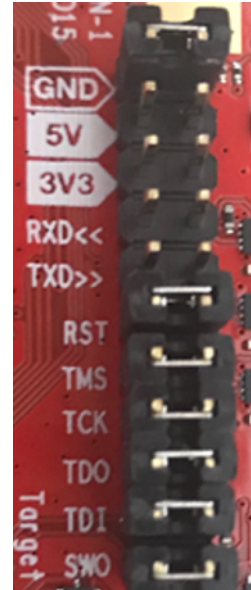
Figure 21. After Removing Four Jumpers
