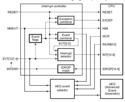
The figure below shows a logical representation of the Event Combiner in the Keystone CorePac. The 124 system events are divided into 4 groups, as shown in the figure below. The Event Combiner logic has the capability of grouping multiple event inputs to 4 possible event outputs, EVT[3:0]. These outputs are then provided as inputs to the interrupt selector and treated as additional system events. This is illustrated in the figure above [2]
