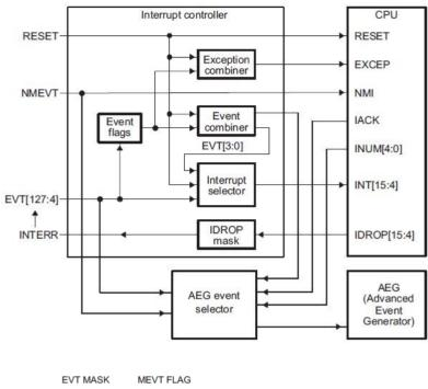
The figure below shows a logical representation of the Event Combiner in the Keystone CorePac. The 124 system events are divided into 4 groups, as shown in the figure below. The Event Combiner logic has the capability of grouping multiple event inputs to 4 possible event outputs, EVT[3:0]. These outputs are then provided as inputs to the interrupt selector and treated as additional system events. This is illustrated in the figure above [2]
