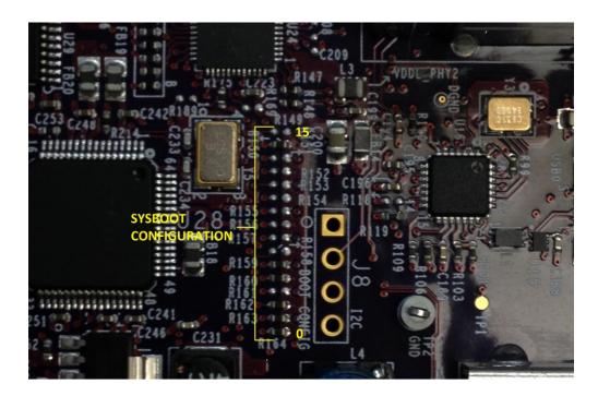
On the General purpose EVM, the SYSBOOT pins can be freely configured using the SYSBOOT Dip Switches (SW3+SW4). The Dip switches and their relation to the SYSBOOT pins can be seen below.
