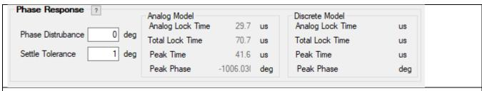
The phase response box models the phase of the output and lock time to a phase. A nonzero entry for the Phase Disturbance can be given to model a step response in phase and this is shown in the graph on the lower left.
