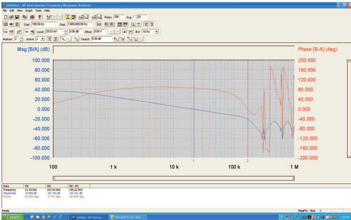
Figure 8. Bode Plot for TPS53219EVM With All-Ceramic Capacitor Application
