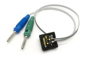
Figure 11: Positive input (+) blue and negative input (-) green. The colour coding matches the outputs of Amalthea
