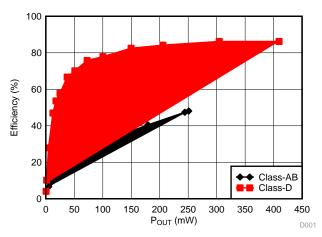
Figure 23. Efficiency Graphs of the TPA731 and TPA2001D1
