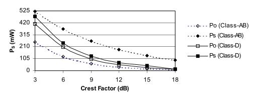
Figure 25. Supply and Output Power Versus CF for the TPA731 and TPA2001D1
