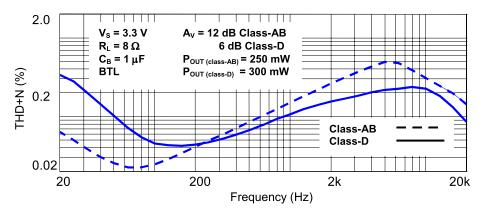
Figure 10. THD+N Versus Frequency for the TPA2001D1 and the TPA731
