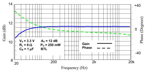
Figure 14. TPA731 Gain and Phase Measurements
