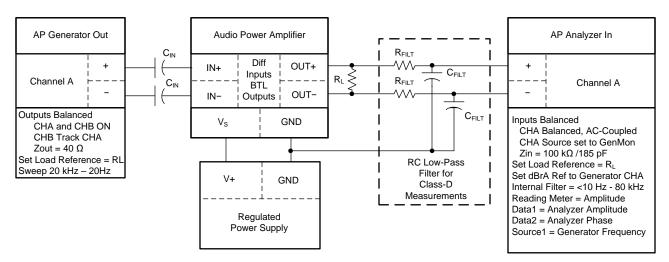
Figure 13. Gain and Phase Measurement Circuit
