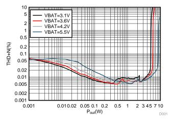
Figure 8. THD+N Versus POUT for the TAS2562. 4- $\Omega$  load. 1 KHz.
