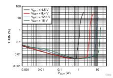
Figure 7. THD+N Versus POUT for the TAS2770. 8- $\Omega$  Load. 1 KHz.
