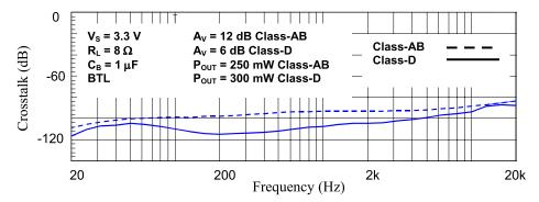
Figure 17. Crosstalk Measurements
