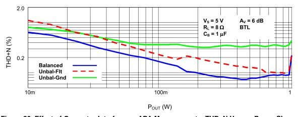
Figure 26. Effect of Generator Interface on APA Measurements, THD+N Versus Power Shown
