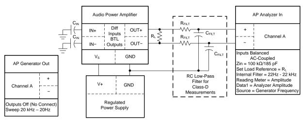
Figure 11. Noise Measurement Circuit
