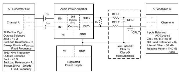
Figure 5. THD+N Measurement Circuit Using the AP-II Measurement System: Differential-BTL
