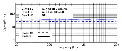
Figure 12. Measured Results of Noise Circuit
