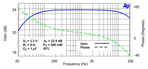
Figure 15. TPA2001D1 Gain and Phase Measurements
