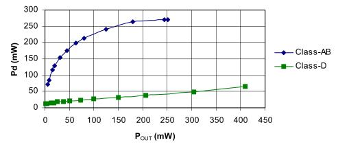
Figure 24. Graph of Power Dissipated Versus Output Power
