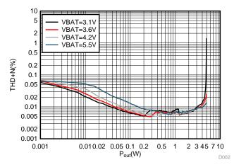
Figure 9. THD+N Versus POUT for the TAS2562. 4- $\Omega$  Load. 1 KHz.
