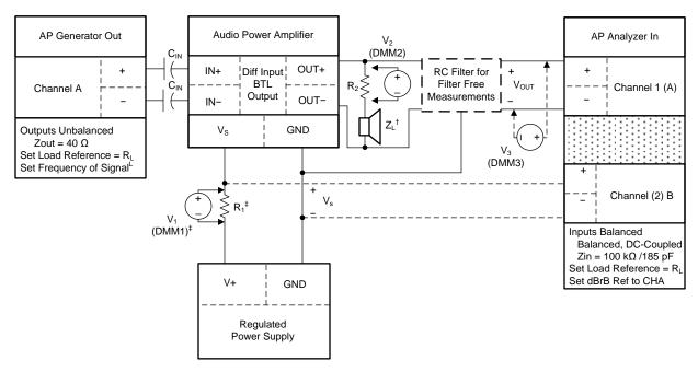
$\dagger$  Load  $Z_L$  is a speaker for class-D APAs and is a purely resistive load for class-AB APAs
