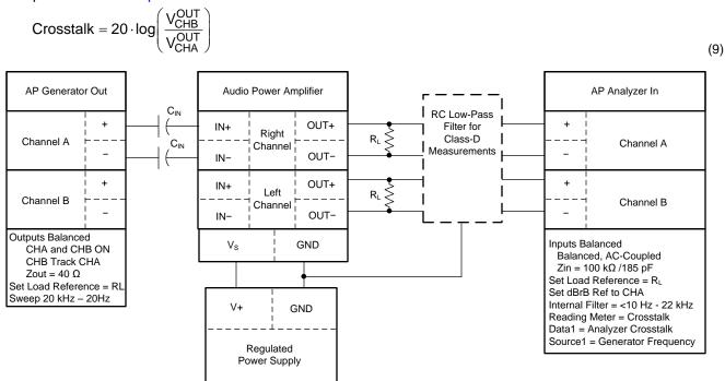
Figure 16. Crosstalk Measurement Circuit
