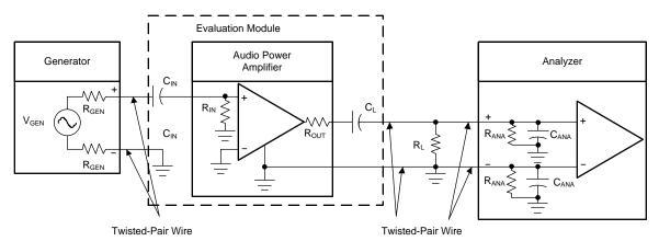
Figure 3. SE Input—SE Output Measurement Circuit
