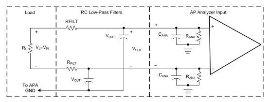
Figure 4. Measurement Low-Pass Filter Derivation Circuit—Class-D APAs
