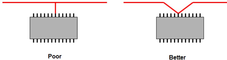
Figure 9. Avoid Right-Angle Traces
