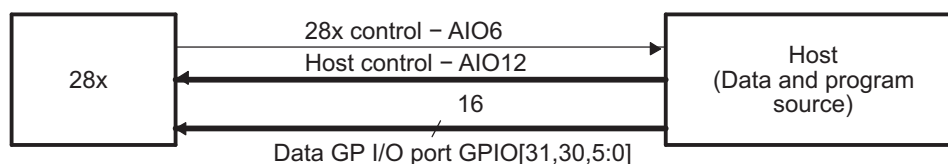
Figure 14. Overview of Parallel GPIO bootloader Operation
