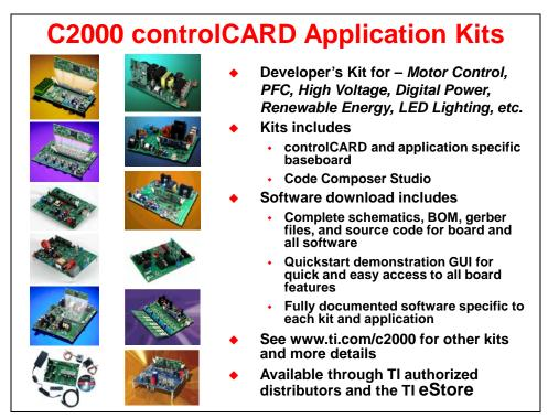
The controlCARD based Application Kits demonstrate the full capabilities of the C2000 device in an application. All kits are completely open source with full documentation.
