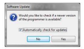
If the "Automatically check for updates" option is enabled, the programmer will periodically query the update-server to check if a newer version of the application is available.
