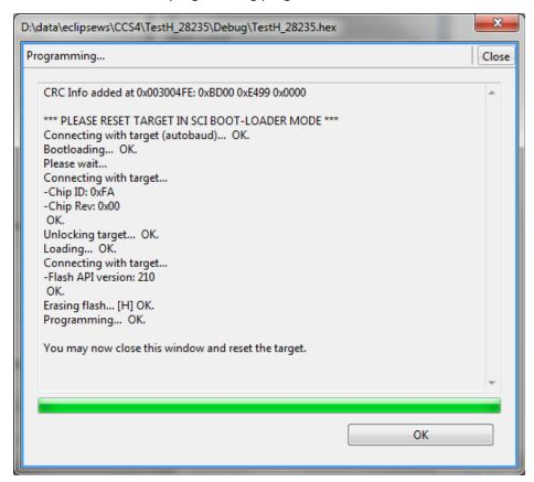
Important: Do not interrupt the programming as this can cause the MCU to be permanently locked.
