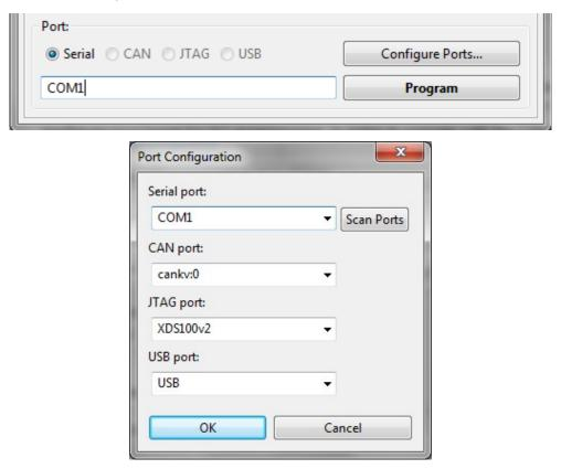
The "Scan Ports" button in the Port Configuration Dialog automatically scans for all available serial ports. Note that on some computers this feature can take a very long time to execute (particularly if Bluetooth COM ports are present).
