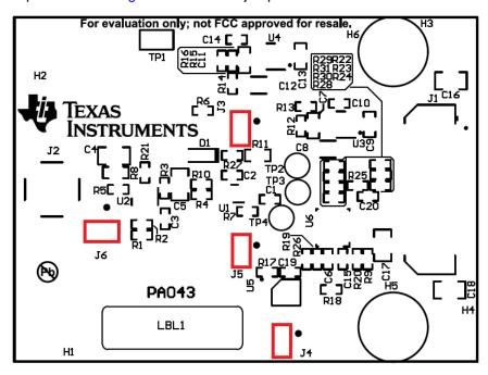
Figure 2. ADS7049-Q1EVM-PDK Jumper Locations
