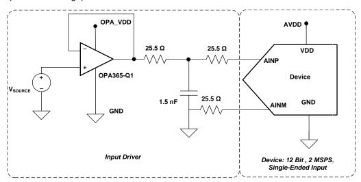
Figure 1. ADS7049-Q1EVM Analog Input Path
