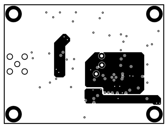
Figure 16. ADS7049-Q1EVM PCB Layer 3: Power Planes
