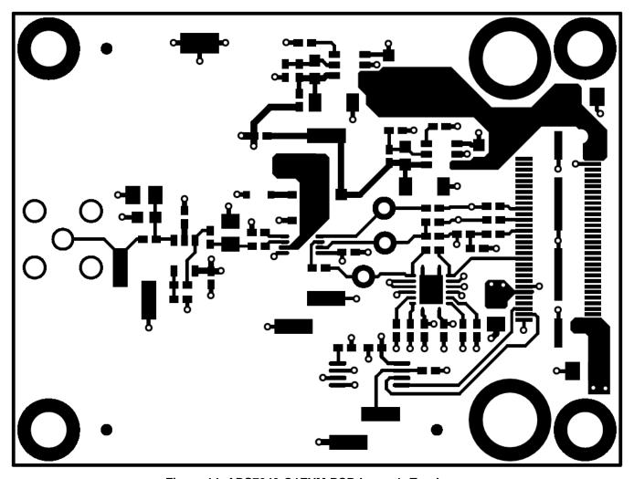
Figure 14. ADS7049-Q1EVM PCB Layer 1: Top Layer
