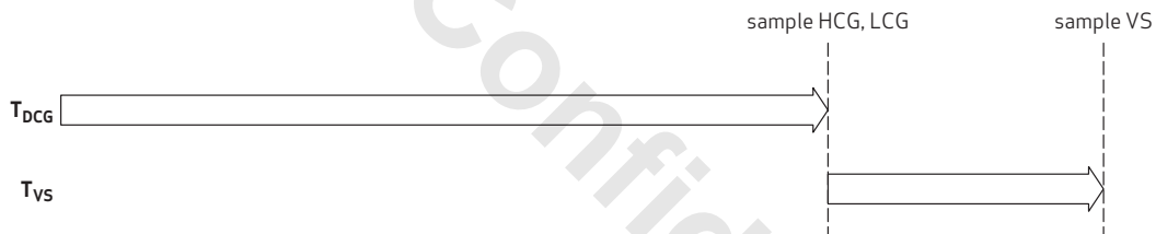
figure 3-4 integration time diagram for dual exposure staggered HDR mode
