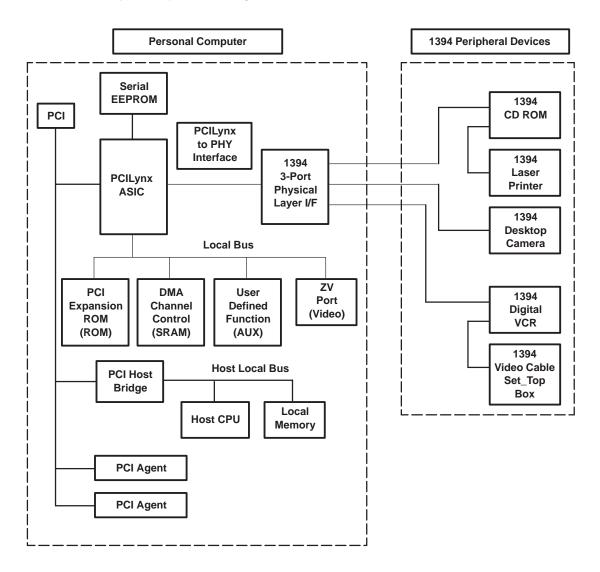
Figure 1. PCILynx ASIC in a Typical System Configuration
