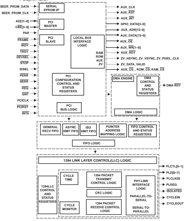
Figure 2. PCILynx Functional Partitioning
