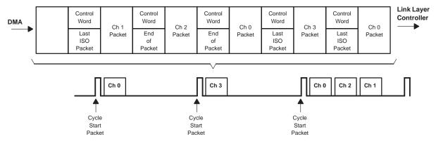
Figure 10. Isochronous Transmit Packet Framing
