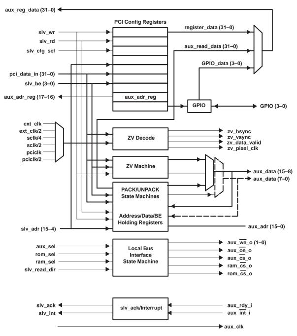
Figure 4. Local Bus Interface Block Diagram
