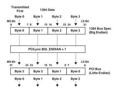
Figure 6. 1394 Data Byte Addressing not Preserved on the PCI Bus
