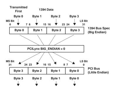
Figure 5. 1394 Data Byte Addressing is Preserved on the PCI Bus
