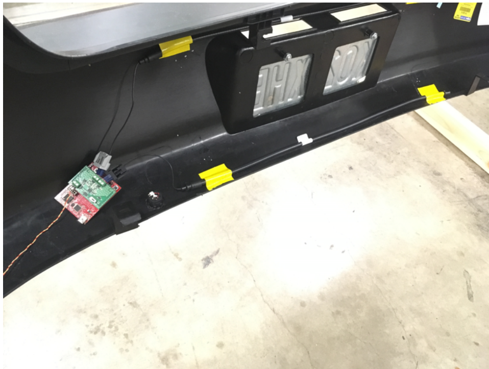
Figure 20. Capacitive Antennas Mounted on Bumper Cover
