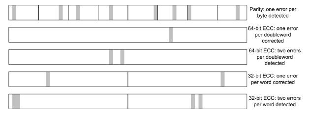
Figure 8-2 Error detection and correction schemes
