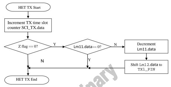
Figure 2. N2HET Emulated UART Transmit Program FlowChart
