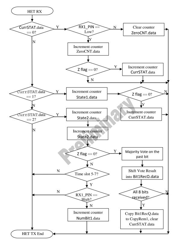
Figure 4. N2HET Emulated UART Receive Program FlowChart
