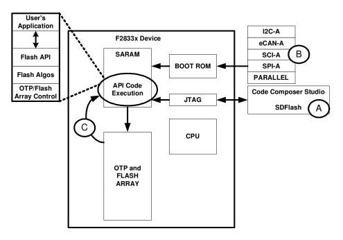
Method A: The code is loaded directly into on-chip SARAM via the JTAG port. This is the method used by Code Composer Studio and the SDFlash utility.
