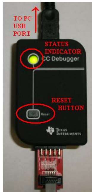
Figure 42 CC Debugger Interface
