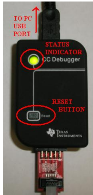
Figure 46 CC Debugger Interface
