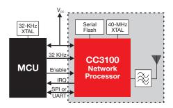
easily to any low-cost and low-power micro-controller (MCU) such as the MSP430F5529 or MSP430FR5969, due to a simple UART or SPI driver and host memory footprint as low as 7kB of code to reside on the MCU. Hardware design flexibility includes a 64-pin 9×9 mm QFN package or upcoming certified CC3100 module. Flexible connection methods (provisioning)
