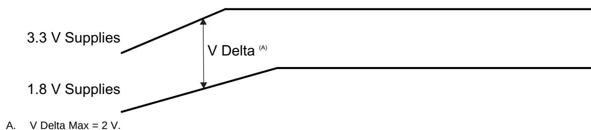
Figure 7-2. 3.3 V Supplies Rising Before 1.8 V Supplies Delta
