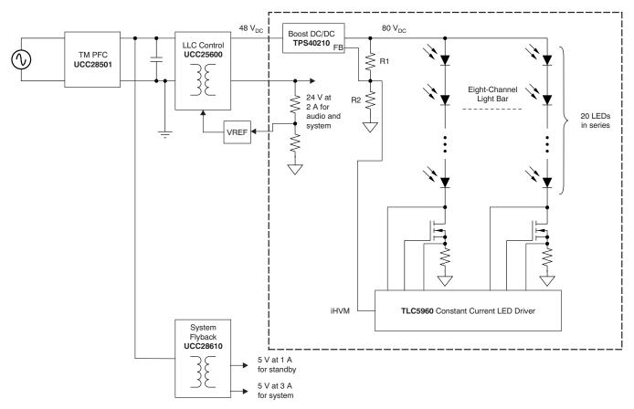
Figure 2. PMP4298: Basic Architecture for LED Backlight LCD TV Power Supply
