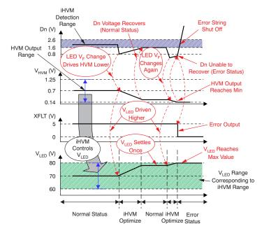
Figure 9. LED Open Detection and V<sub>LED</sub> Optimization Through iHVM
