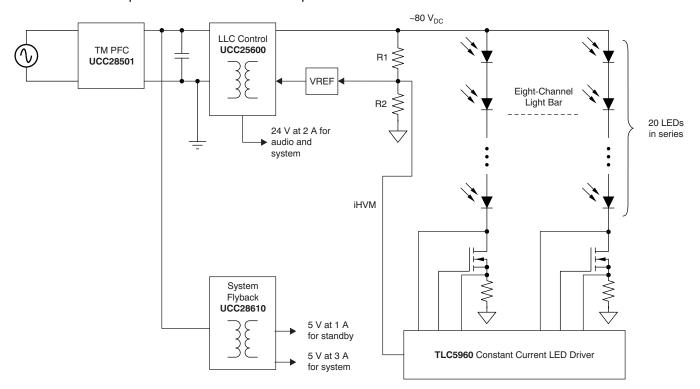
Figure 3. PMP4298A: Advanced Power Architecture for LED Backlight LCD TV
