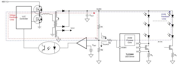
Figure 6. AC-DC Power-Stage Direct Feedback Loop Integrated with iHVM Secondary Feedback
