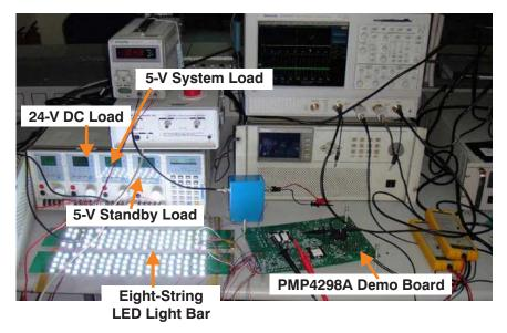
Figure 11. PMP4298A Demonstration Fixture Test Setup
