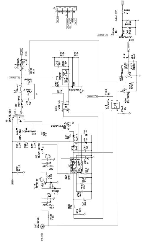
Figure 17. Auxiliary Flyback Converter Stage Schematic for PMP4298 and PMP4298A
