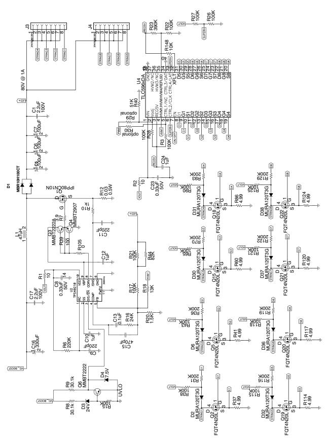
Figure 20. TLC5960 LED Driver Stage Schematic for PMP4298
