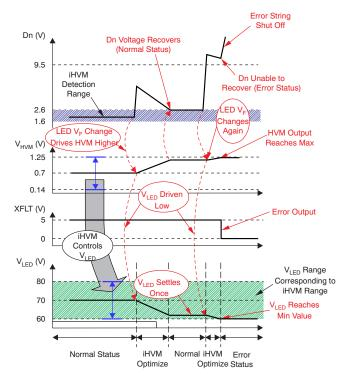
Figure 10. LED Short Detection and  $V_{\mbox{\tiny LED}}$  Optimization Through iHVM
