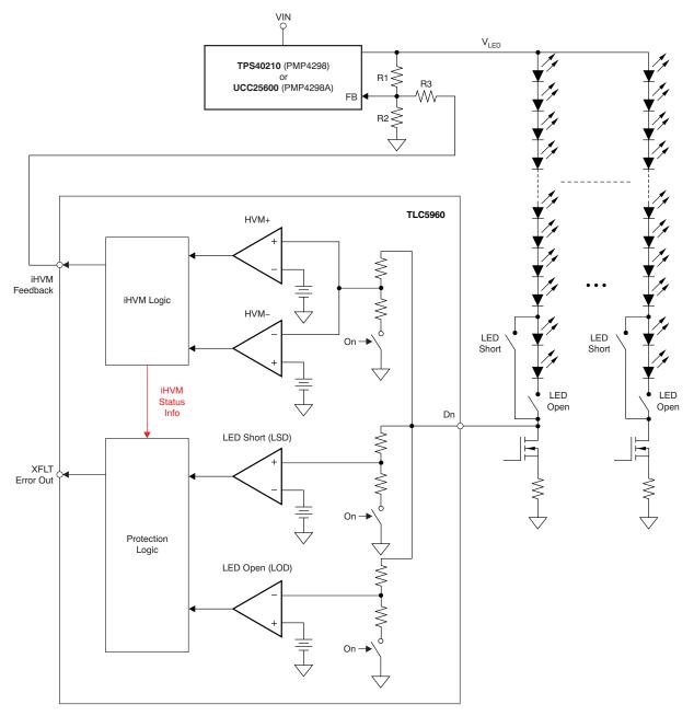
Figure 8. TLC5960 Total iHVM and Protection Scheme
