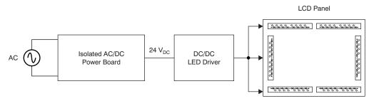
Figure 1. Edge-Type LED Backlight LCD TV Power Conversion Scheme
