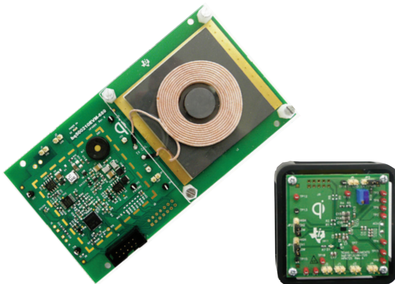
Development kit includes bq500210 and bq51013 evaluation modules.
