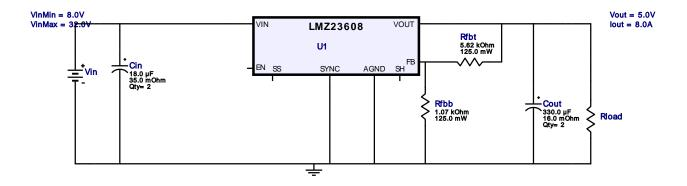
1. This design cannot function without airflow at maximum input voltage and full load current. An airflow of 225LFM is required to bring down the ThetaJA of the IC.
