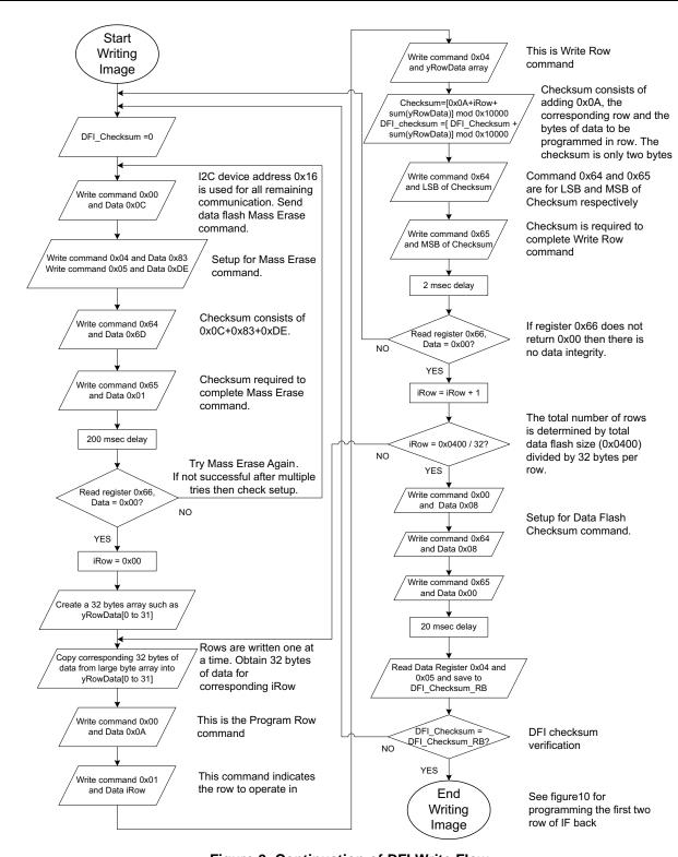
Figure 9. Continuation of DFI Write Flow
