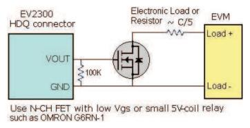
Figure 5. Load Connection for Automated Discharge
