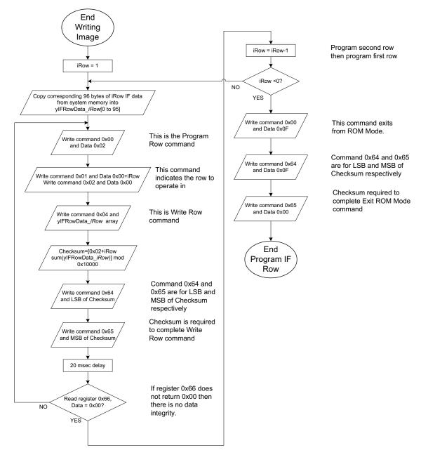
Figure 10. Continuation of DFI Write Flow
