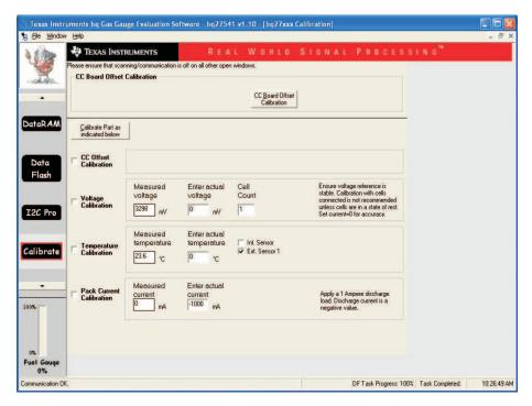
Figure 3. bq27541 EVSW Calibration Screen
