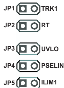
Figure 6. Configure the EVM as a Master for Stackable Operation
