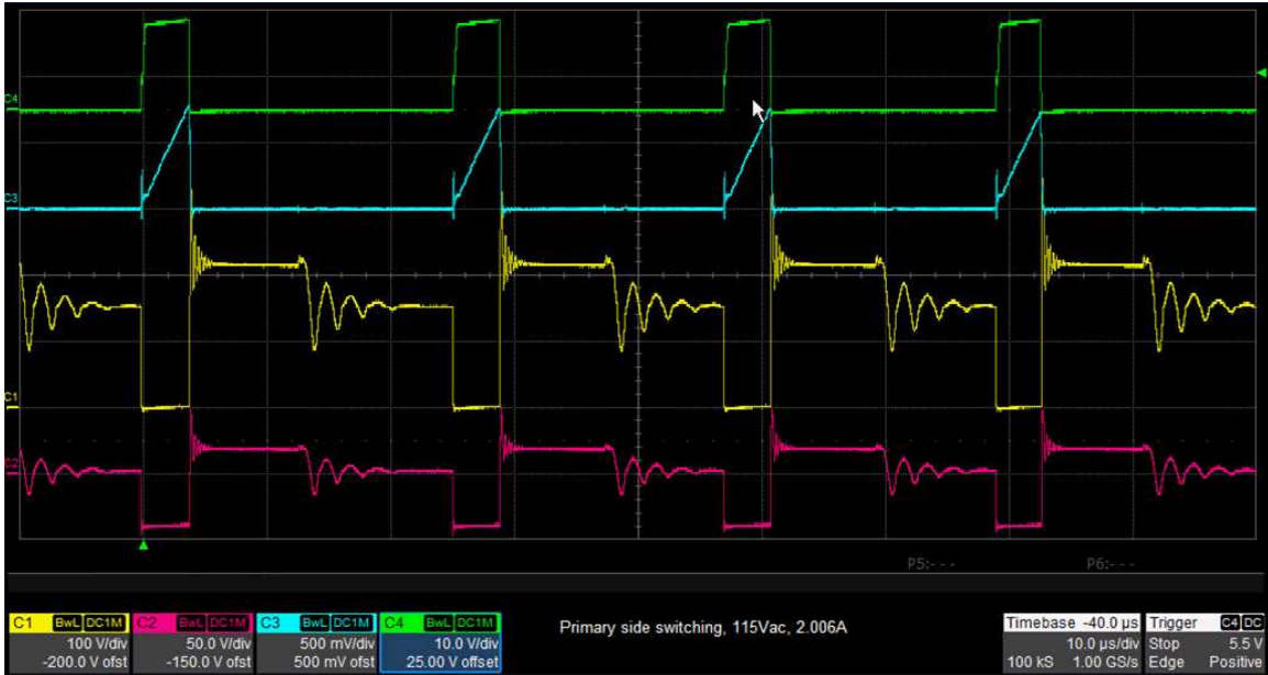
Figure 14. Primary-Side Switching Waveform
