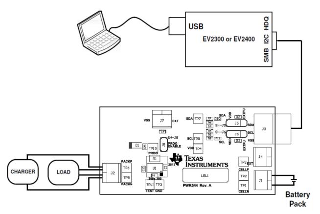
Figure 5. bq27411 Circuit Module Connection to Pack and System Load/Charger
