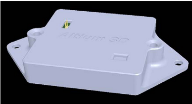
Figure 13. Multivibrator PCB fully assembled into two part housing assembly.
