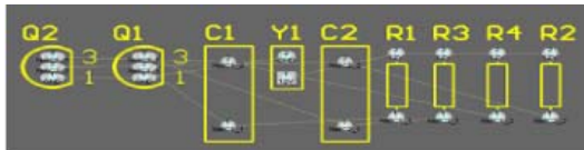
Figure 4. The components next to the board, ready for positioning.
