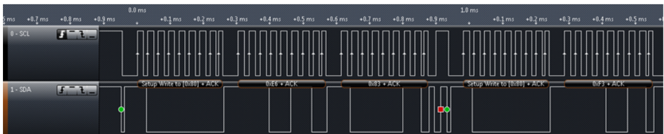
Figure 18. I2C Set Up and Start Temperature Measurement
