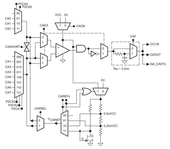
Figure 21-1. Comparator\_A+ Block Diagram
