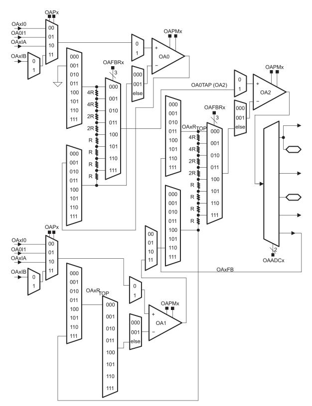
Figure 20-5. Three-Opamp Differential Amplifier OAx Interconnections
