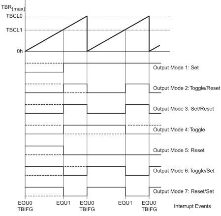
Figure 13-12. Output Example, Timer in Up Mode
