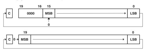
Figure 4-52. Rotate Right Unsigned RRUM[.W] and RRUM.A
