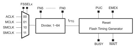
Figure 7-3. Flash Memory Timing Generator Block Diagram
