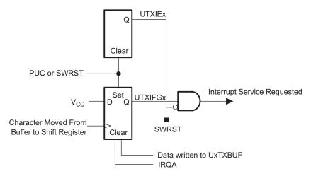
Figure 18-10. Transmit Interrupt Operation
