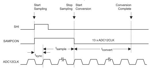
Figure 23-4. Pulse Sample Mode
