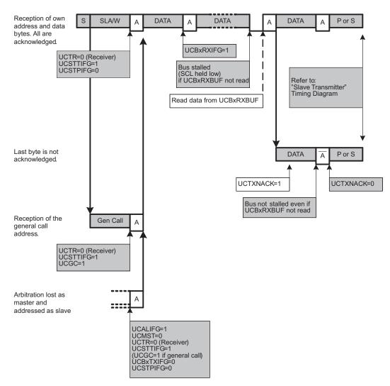
Figure 17-10. I<sup>2</sup>C Slave Receiver Mode
