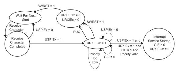
Figure 19-12. Receive Interrupt State Diagram
