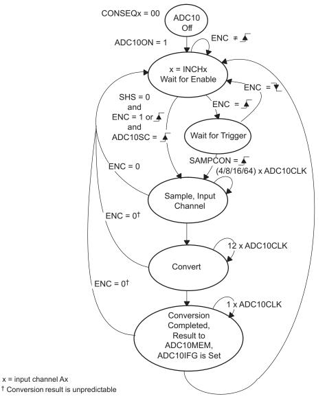
Figure 22-5. Single-Channel Single-Conversion Mode
