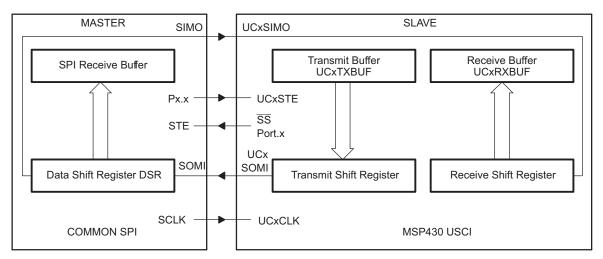
Figure 16-3. USCI Slave and External Master
