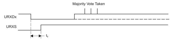
Figure 15-9. Glitch Suppression, USCI Activated
