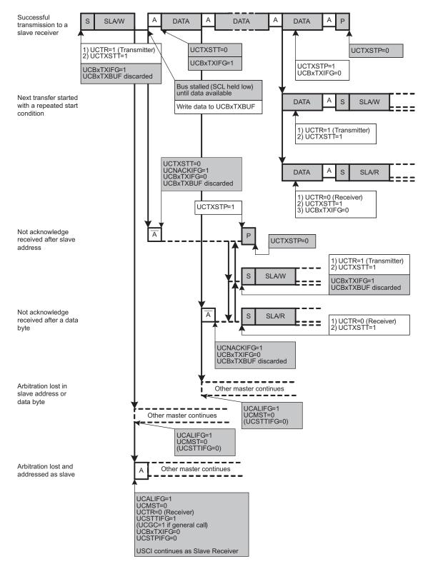
Figure 17-12. I<sup>2</sup>C Master Transmitter Mode
