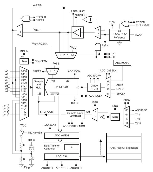
†Channels A12-A15 are available in MSP430F22xx devices only. Channels A12-A15 tied to channel A11 in other devices. Not all channels are available in all devices.
