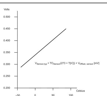
Figure 26-8. Typical Temperature Sensor Transfer Function
