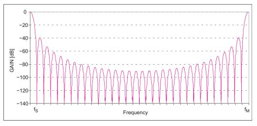
Figure 26-3. Comb Filter Frequency Response With OSR = 32
