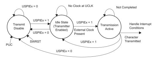
Figure 19-5. Slave Transmit Enable State Diagram
