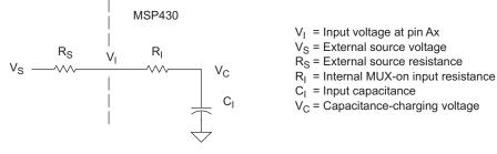
Figure 23-5. Analog Input Equivalent Circuit
