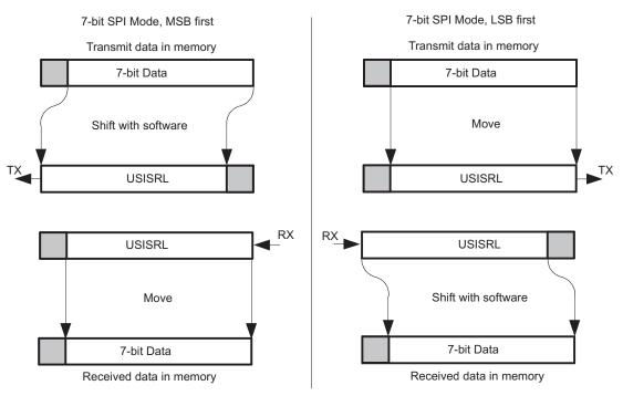
Figure 14-4. Data Adjustments for 7-Bit SPI Data
