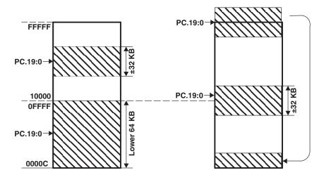
Figure 4-20. Overflow and Underflow for Symbolic Mode
