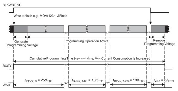
Figure 7-10. Block-Write Cycle Timing
