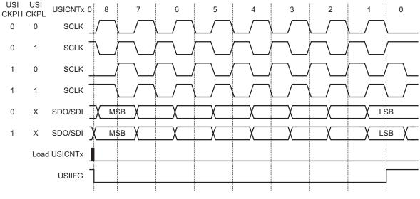
Figure 14-3. SPI Timing
