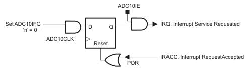
Figure 22-16. ADC10 Interrupt System
