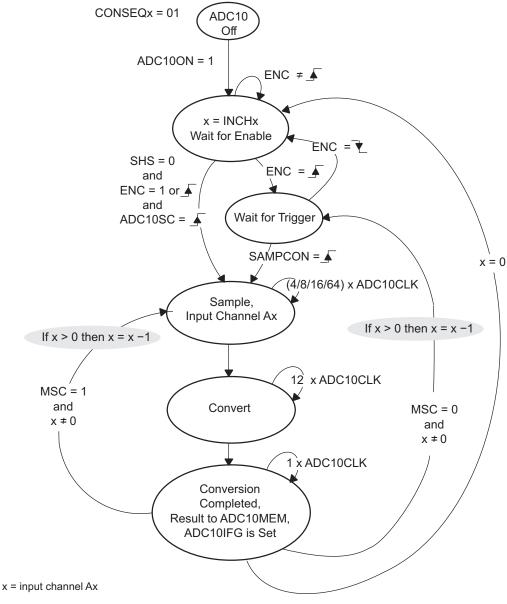
Figure 22-6. Sequence-of-Channels Mode
