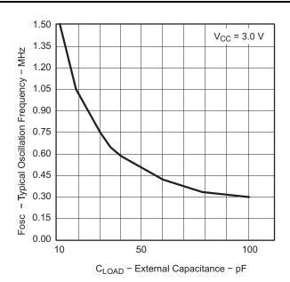
Figure 8-2. Typical Pin-Oscillation Frequency
