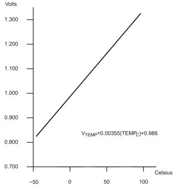
Figure 23-10. Typical Temperature Sensor Transfer Function
