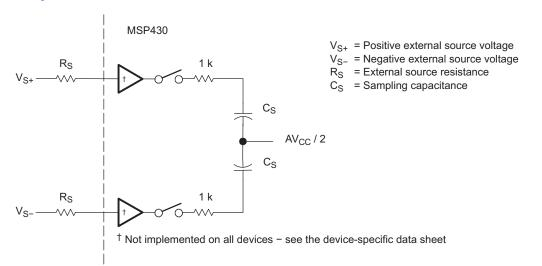
Figure 27-2. Analog Input Equivalent Circuit
