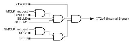
Figure 5-4. Off Signals for Oscillator XT2
