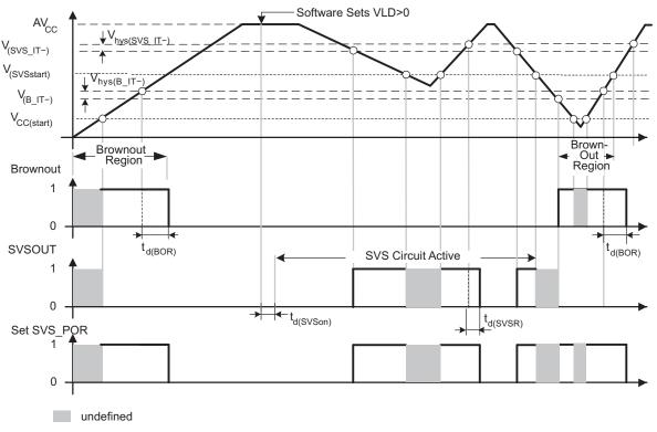
Figure 9-2. Operating Levels for SVS and Brownout/Reset Circuit
