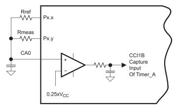
Figure 21-6. Temperature Measurement System
