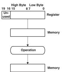
Figure 4-11. Register-Word Operation
