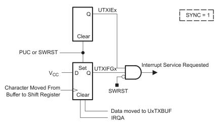
Figure 19-10. Transmit Interrupt Operation
