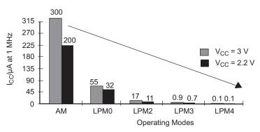
Figure 2-8. Typical Current Consumption of 'F21x1 Devices vs Operating Modes
