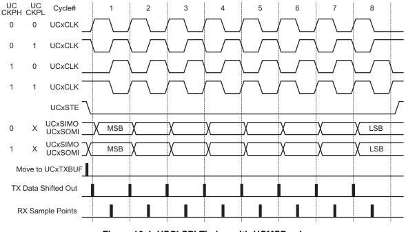
Figure 16-4. USCI SPI Timing with UCMSB = 1
