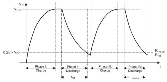
Figure 21-7. Timing for Temperature Measurement Systems
