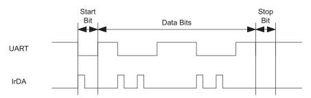
Figure 15-7. UART vs IrDA Data Format
