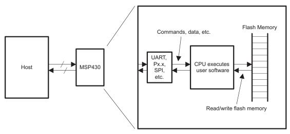
Figure 7-12. User-Developed Programming Solution
