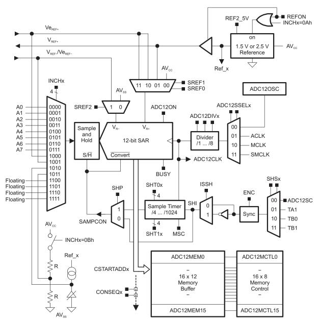
Figure 23-1. ADC12 Block Diagram
