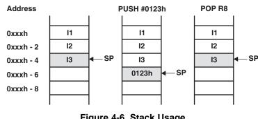
Figure 4-5. Stack Pointer
