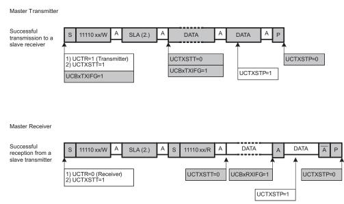
Figure 17-14. I<sup>2</sup>C Master 10-bit Addressing Mode
