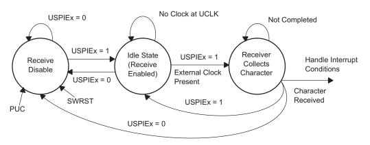
Figure 19-7. SPI Slave Receive-Enable State Diagram
