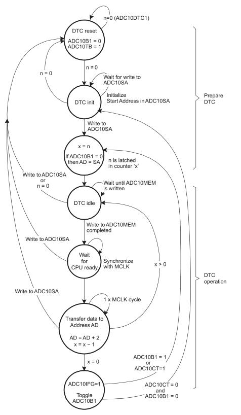
Figure 22-12. State Diagram for Data Transfer Control in Two-Block Transfer Mode
