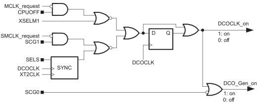
Figure 5-5. On/Off Control of DCO
