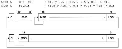
Figure 4-46. Rotate Right Arithmetically RRAM[.W] and RRAM.A
