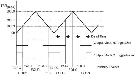
Figure 13-9. Output Unit in Up/Down Mode
