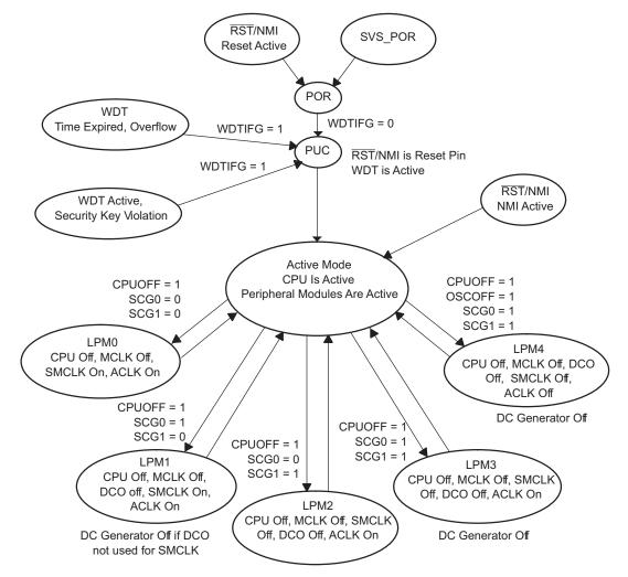
Figure 2-9. Operating Modes For Basic Clock System
