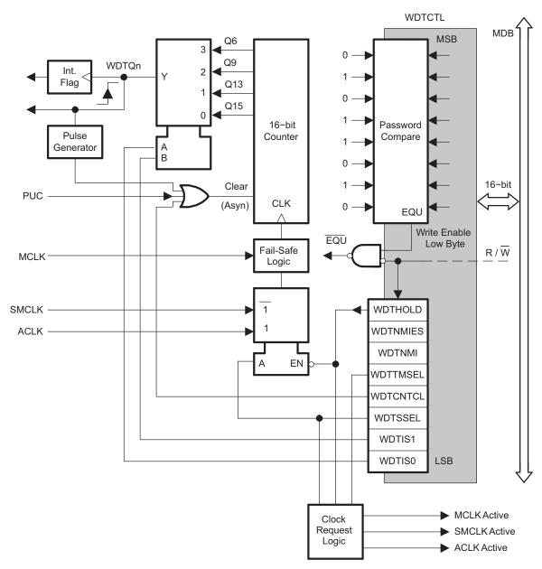
Figure 10-1. Watchdog Timer+ Block Diagram
