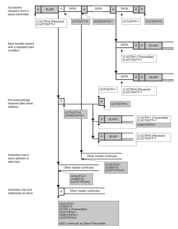
Figure 17-13. I<sup>2</sup>C Master Receiver Mode
