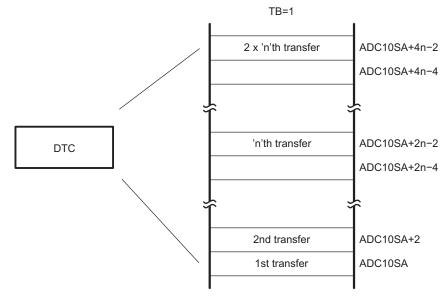
Figure 22-11. Two-Block Transfer
