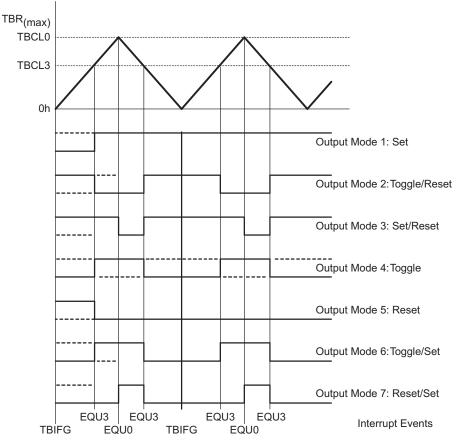
Figure 13-14. Output Example, Timer in Up/Down Mode
