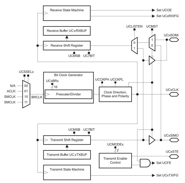
Figure 16-1. USCI Block Diagram: SPI Mode
