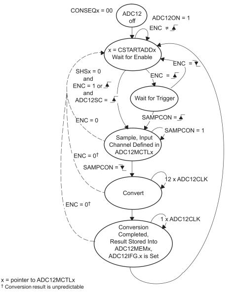
Figure 23-6. Single-Channel, Single-Conversion Mode
