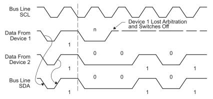
Figure 17-15. Arbitration Procedure Between Two Master Transmitters
