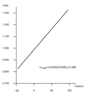
Figure 22-13. Typical Temperature Sensor Transfer Function
