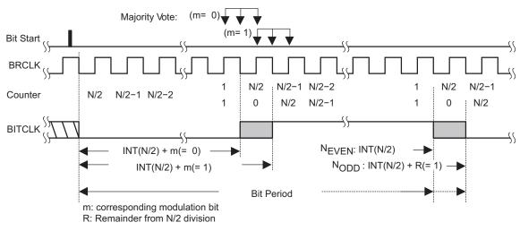
Figure 18-8. BITCLK Baud Rate Timing
