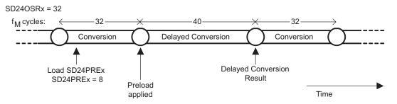
Figure 27-9. Conversion Delay Using Preload - Example
