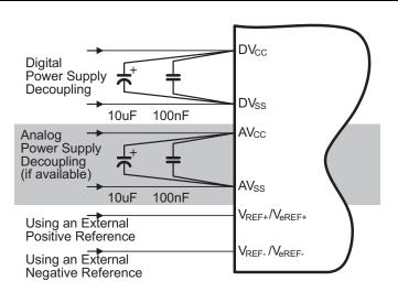
Figure 22-15. ADC10 Grounding and Noise Considerations (External V<sub>REF</sub>)
