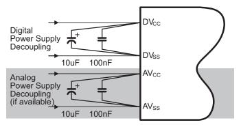
Figure 22-14. ADC10 Grounding and Noise Considerations (Internal V<sub>REF</sub>)
