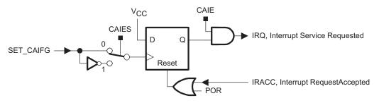
Figure 21-5. Comparator\_A+ Interrupt System
