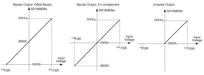
Figure 26-6. Input Voltage vs Digital Output
