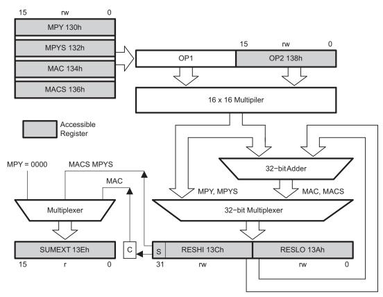
Figure 11-1. Hardware Multiplier Block Diagram
