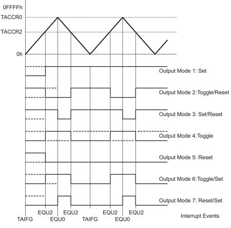
Figure 12-14. Output Example—Timer in Up/Down Mode
