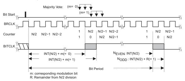
Figure 15-10. BITCLK Baud Rate Timing With UCOS16 = 0
