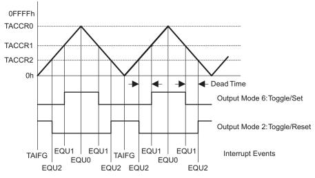
Figure 12-9. Output Unit in Up/Down Mode
