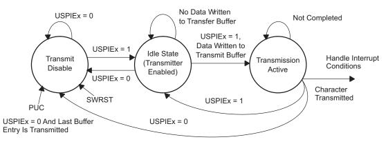
Figure 19-4. Master Transmit Enable State Diagram
