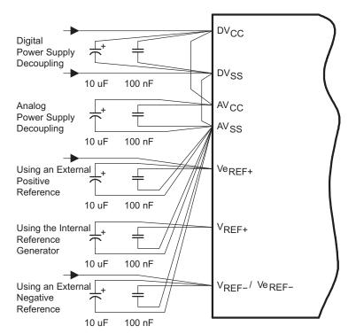
Figure 23-11. ADC12 Grounding and Noise Considerations
