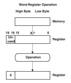
Figure 4-12. Word-Register Operation
