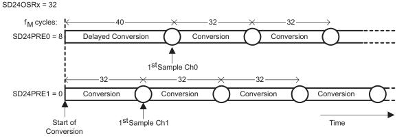
Figure 27-10. Start of Conversion Using Preload - Example
