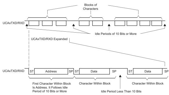
Figure 15-3. Idle-Line Format
