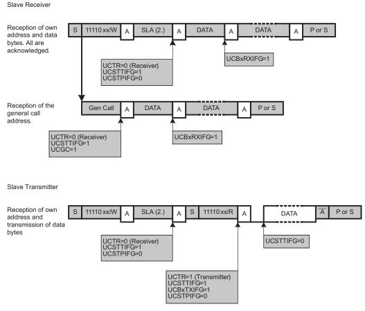
Figure 17-11. I<sup>2</sup>C Slave 10-bit Addressing Mode
