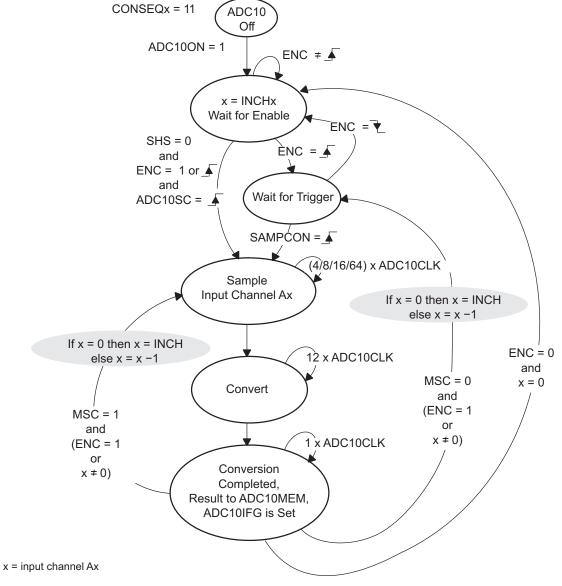
Figure 22-8. Repeat-Sequence-of-Channels Mode
