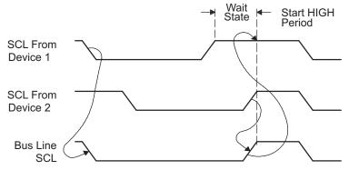
Figure 17-16. Synchronization of Two I<sup>2</sup>C Clock Generators During Arbitration
