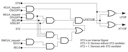
Figure 5-3. Off Signals for the LFXT1 Oscillator
