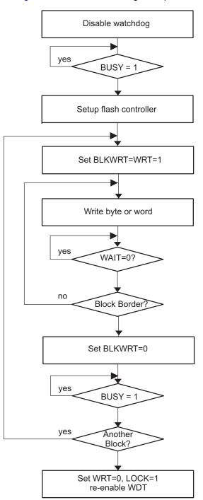
Figure 7-11. Block Write Flow
