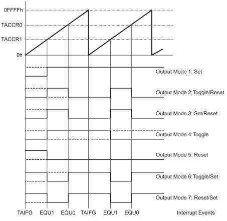
Figure 12-13. Output Example—Timer in Continuous Mode
