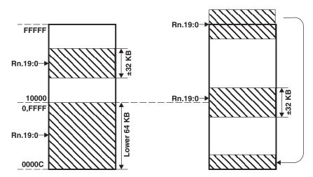
Figure 4-17. Overflow and Underflow for Indexed Mode
