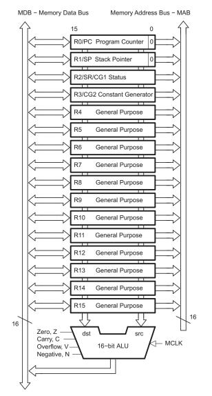
Figure 3-1. CPU Block Diagram
