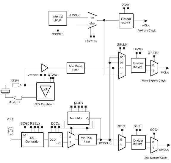
Figure 5-2. Basic Clock Module+ Block Diagram - MSP430AFE2xx
