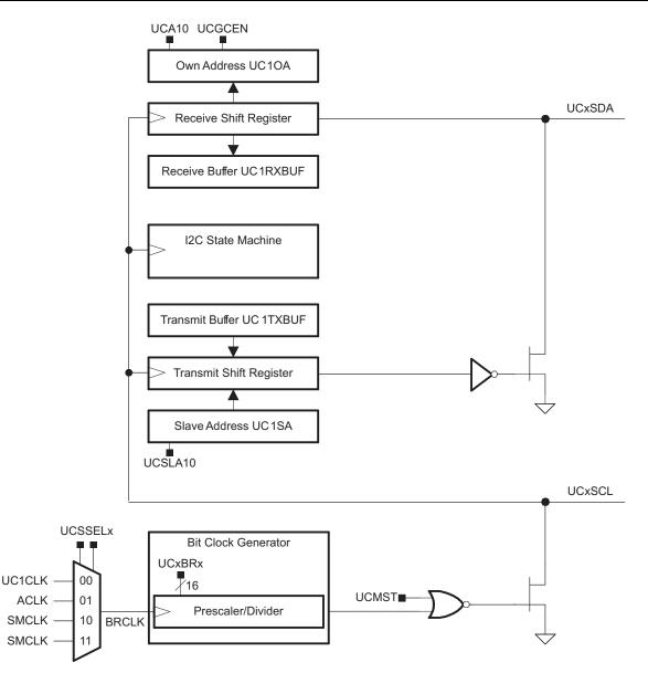
Figure 17-1. USCI Block Diagram: I<sup>2</sup>C Mode
