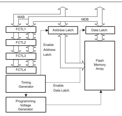
Figure 7-1. Flash Memory Module Block Diagram
