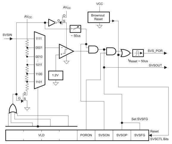
Figure 9-1. SVS Block Diagram
