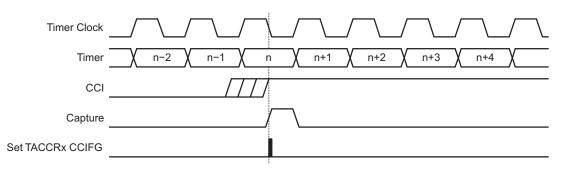
Figure 12-10. Capture Signal (SCS = 1)
