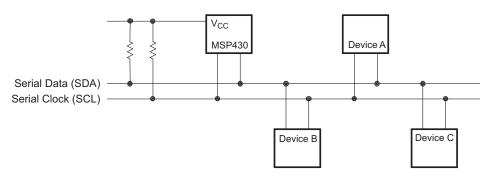
Figure 17-2. I<sup>2</sup>C Bus Connection Diagram
