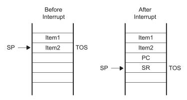
Figure 2-6. Interrupt Processing
