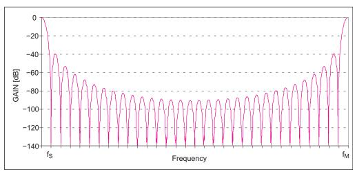
Figure 27-3. Comb Filter Frequency Response With OSR = 32
