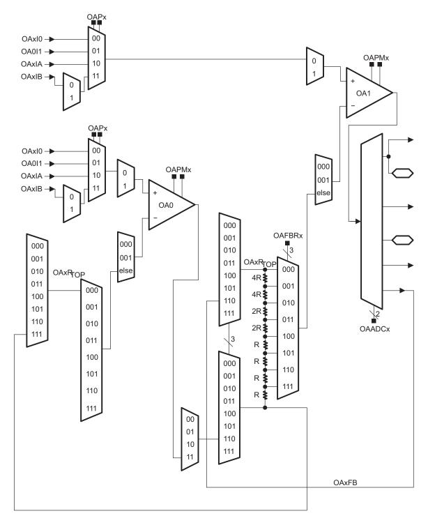
Figure 20-3. Two-Opamp Differential Amplifier OAx Interconnections
