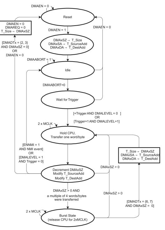
Figure 6-5. DMA Burst-Block Transfer State Diagram
