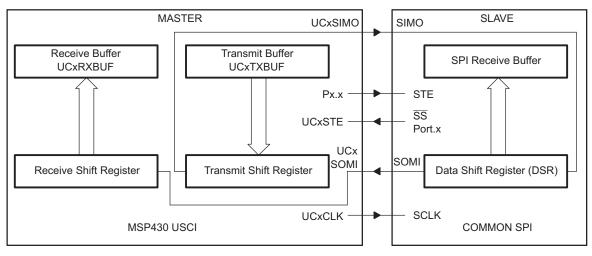
Figure 16-2. USCI Master and External Slave
