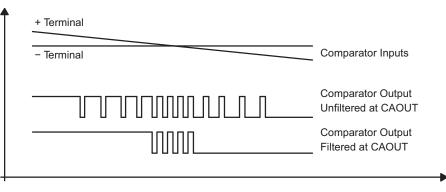
Figure 21-3. RC-Filter Response at the Output of the Comparator
