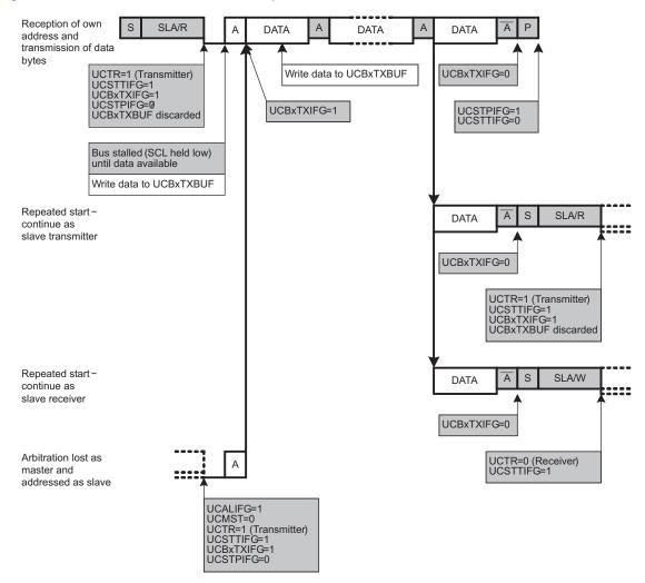
Figure 17-9. I<sup>2</sup>C Slave Transmitter Mode
