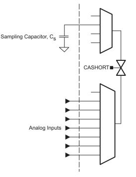
Figure 21-2. Comparator\_A+ Sample-And-Hold
