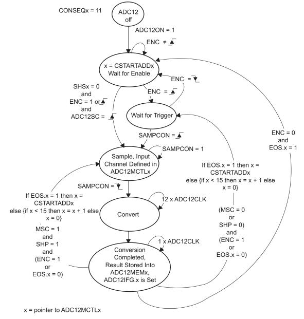
Figure 23-9. Repeat-Sequence-of-Channels Mode
