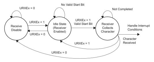
Figure 18-5. State Diagram of Receiver Enable
