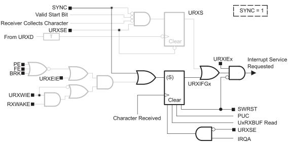
Figure 19-11. Receive Interrupt Operation
