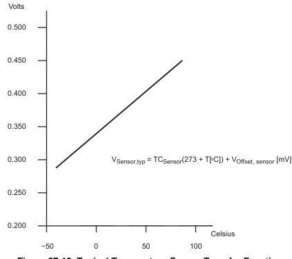
Figure 27-12. Typical Temperature Sensor Transfer Function
