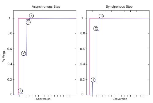
Figure 26-4. Digital Filter Step Response and Conversion Points
