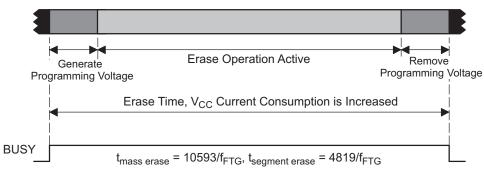
Figure 7-4. Erase Cycle Timing
