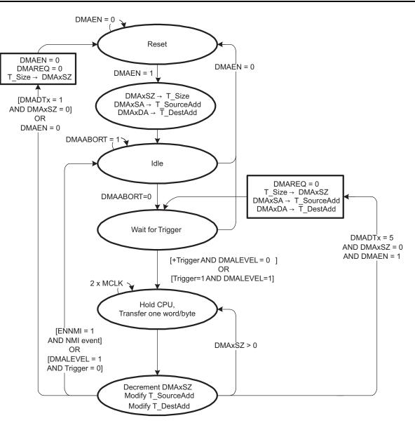
Figure 6-4. DMA Block Transfer State Diagram
