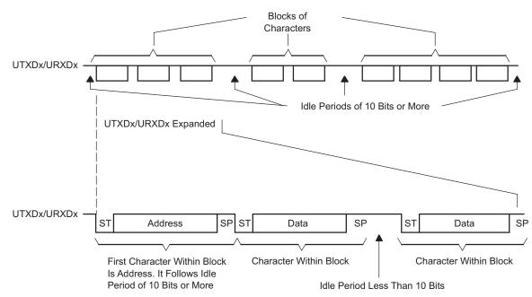
Figure 18-3. Idle-Line Format
