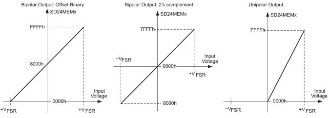
Figure 27-6. Input Voltage vs Digital Output
