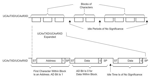
Figure 15-4. Address-Bit Multiprocessor Format
