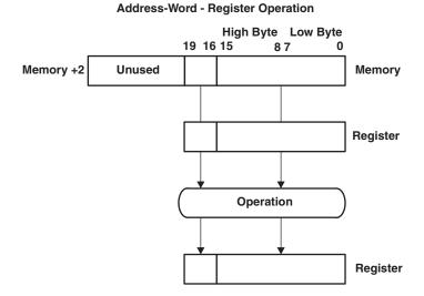
Figure 4-14. Address-Word – Register Operation
