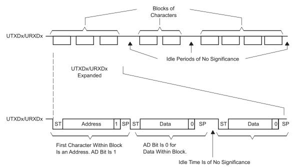
Figure 18-4. Address-Bit Multiprocessor Format
