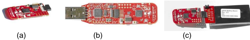
Figure 1: ZNP Mini Kit (a) ZNP Mini Kit Target board (b) eZ430 USB Stick with target board (c) ZNP Mini Kit Battery board
