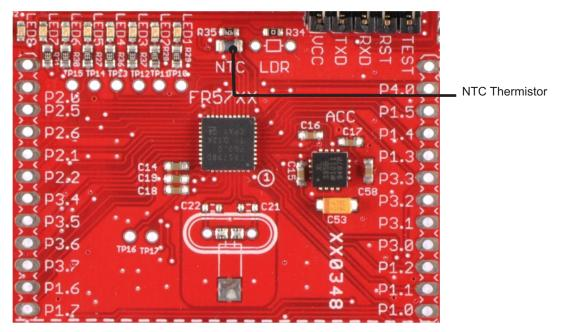
Figure 5. On-Board NTC Thermistor
