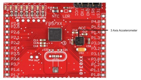
Figure 4. On-Board Accelerometer
