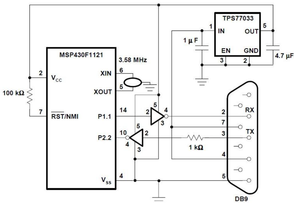
Figure 1. MSP430x11x(1) UART Demonstration Circuit
