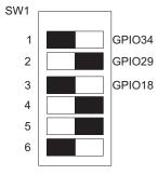
Figure 2. Boot to SARAM Switch 1 Configuration on eZdspF2808
