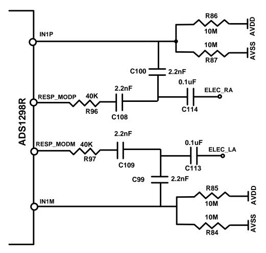
Increasing the input high pass frequency will filter the ECG signal This can be accomplished by reducing C99 and C100
