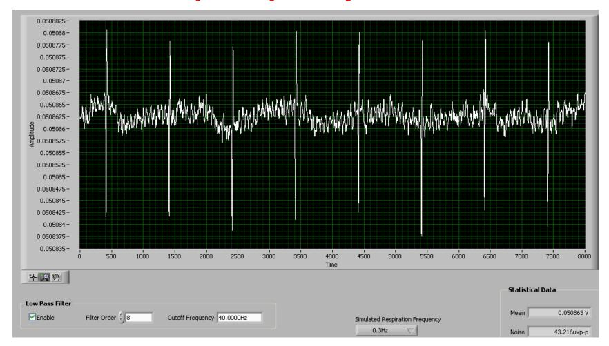
•The respiration signal can still be detected for this case once it is low pass filtered.
