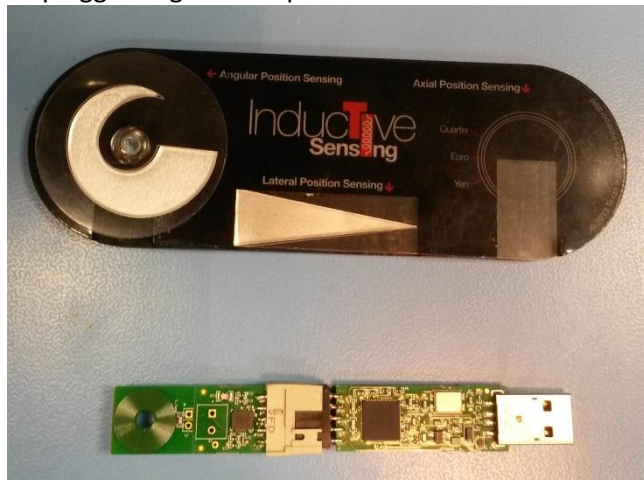
Figure 2 LDC board and MSP-USB board with Inductive Sensing Demonstrator
