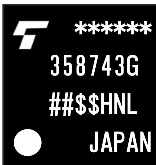
Figure 2.2 Package Marking without HDCP Key, HNL is appended to lot code
