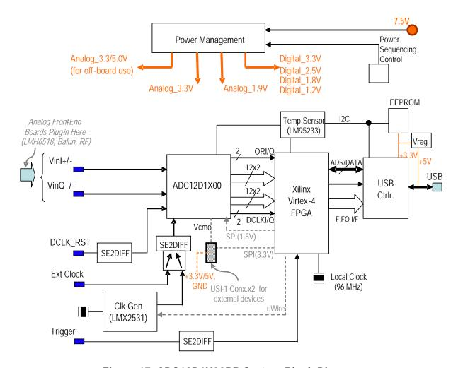
Figure 17: ADC12D1X00RB System Block Diagram
