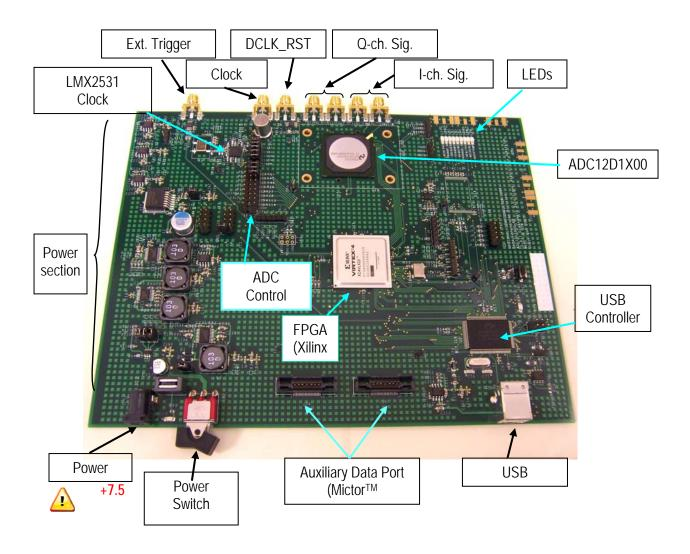
Figure 1: ADC12D1X00RB Board Layout
