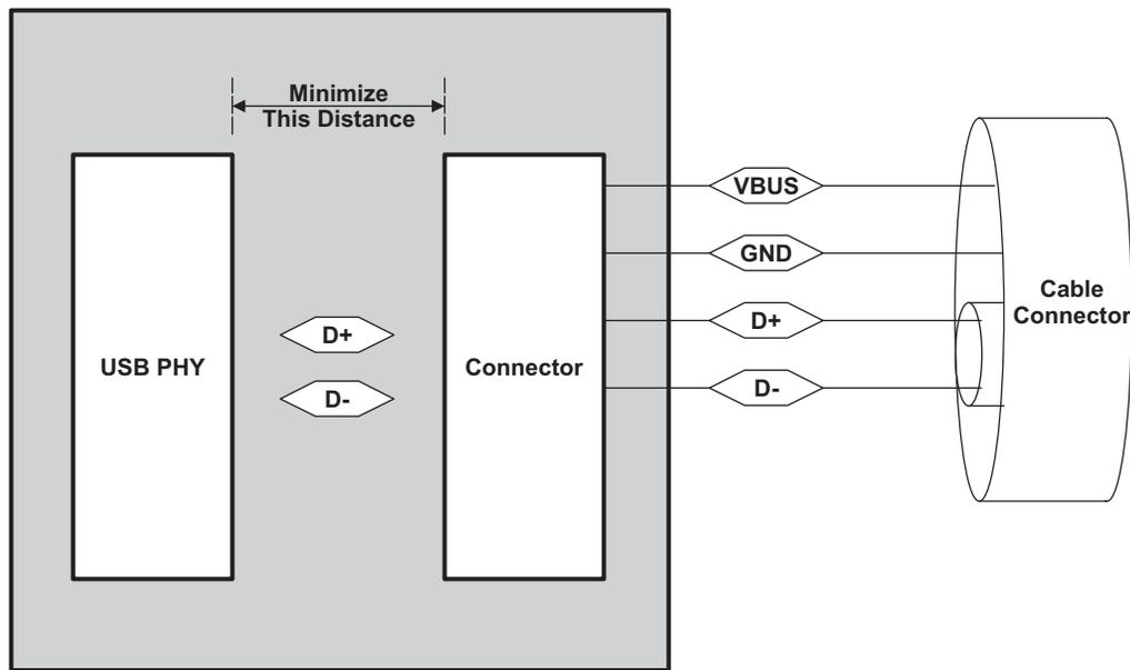
**Figure 6. USB PHY Connector and Cable Connector**
